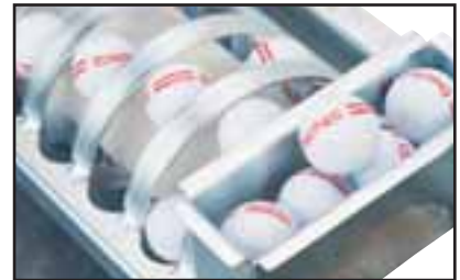
The rotating brush moves the balls through the spiral.
