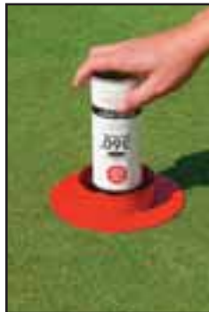
3. Insert spray can into center of painting tool and simply push down on the can 3-4 times. No rotating is necessary.
